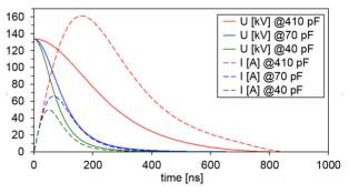
Figure 5: Voltage and current during sparkover.
