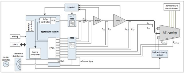
Figure 6: Overview layout of an rf station with digital LLRF system, amplifiers and cavity.
