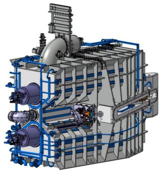
Figure 2: Isometric view of Resonator 4 with tuner, coupling loop in the front and vacuum pump on the top.
