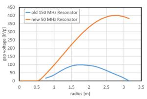
Figure 1: Gap voltage of Resonators 2 & 4.
