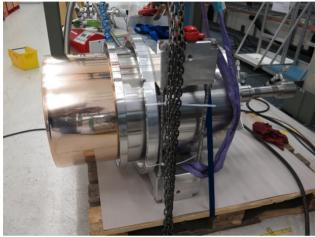
Figure 4: The tuner for the new 50 MHz resonator.
