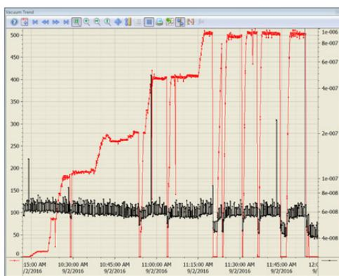
Figure 8: Vacuum and beam current ( $\mu\text{A}$ ) versus time.
