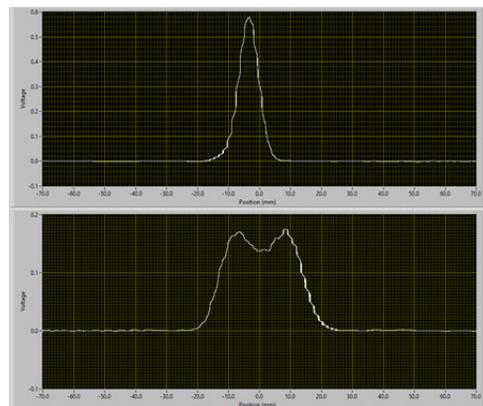
Figure 2: Beam profile (V), wobbler off/on versus  $x$  axis position.
