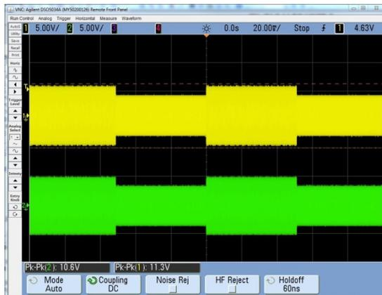
Figure 3: Amplitude modulation (sample) versus time.
