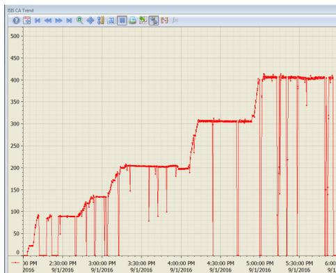
Figure 7: Beam current on target ramp-up ( $\mu\text{A}$ ), versus time.
