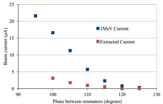
Figure 6: Beam transmission versus phase difference.
