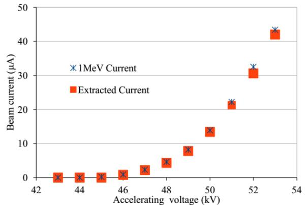
Figure 5: Beam transmission with amplitude.
