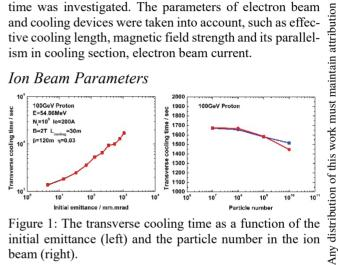
Figure 1: The transverse cooling time as a function of the initial emittance (left) and the particle number in the ion beam (right).
