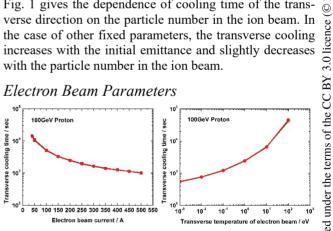
Figure 2: The transverse cooling time as a function of the electron beam current (left) and the transverse temperature of electron beam (right).
