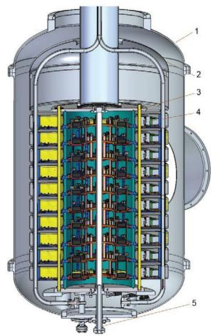
Figure 1: The structure of the high voltage column. 1 – SF<sub>6</sub> tank; 2 – shielding cover; 3 – high voltage cascade transformer; 4 - high voltage section; 5 - isolating and cooling oil tubes.
