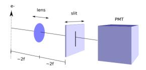
Figure 2: Schematic of the optical setup.
