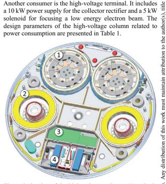
Figure 2: Section of the high-voltage column: (1) a single ring of the cascade transformer, (2) a magnetic coil for creating a guiding magnetic field in the accelerating tube, (3) control electronics, (4) high-voltage power supplies.
