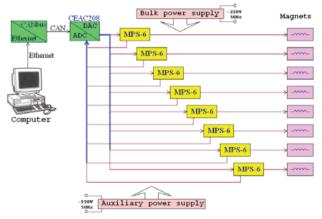
Figure 1: Structure of power module MPS-6.
