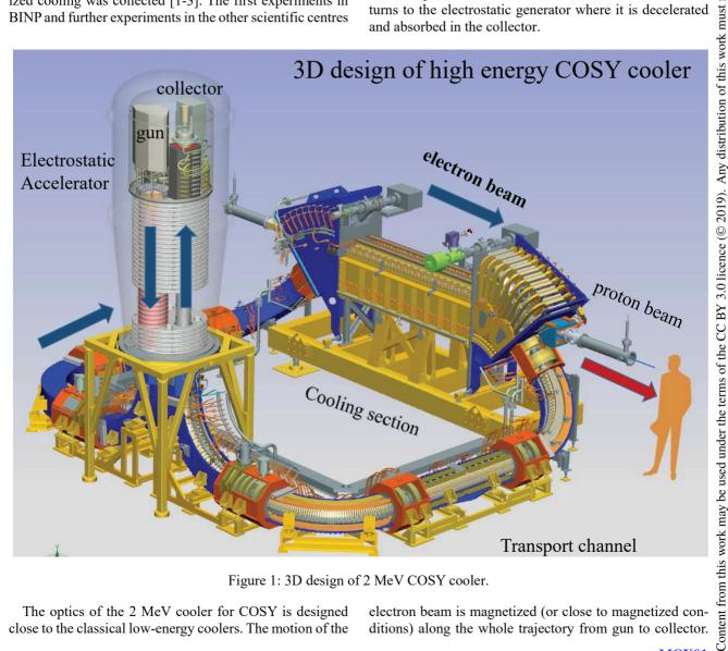
Figure 1: 3D design of 2 MeV COSY cooler.
