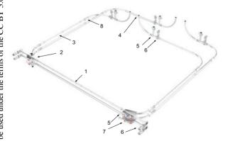
Figure 1: 1 - Cooling section vacuum chamber with BPMs (every one meter), 2 – toroid bend chamber equipped with two 2000 l/s NEG cartridges each, 3 - straight transport channel chamber with BPM, 4 - transition to the electrostatic accelerator, 5 - pumping ports, 6 - gate valves, 7 - NEG cartridges, 8 - special insertion with 1400 1/s NEG cartridge.
