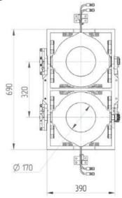
Figure 2: Cooling solenoid cross-section.
