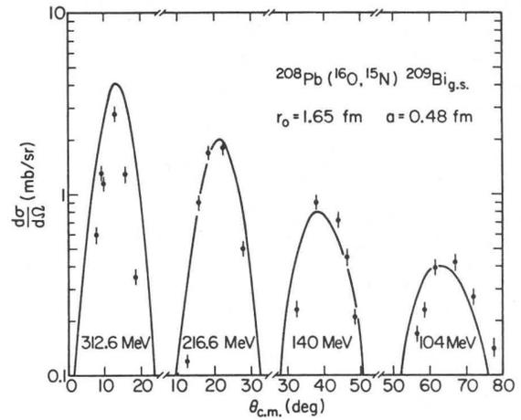
Fig. 3 Differential cross sections for the reaction  $^{208}\text{Pb}(^{16}\text{O},^{15}\text{N})^{209}\text{Bi}$  populating the  $h_{9/2}$  ground state at an incident energy of 104, 140, 216.6 and 312.6 MeV, from right to left. The solid lines are DWBA calculations described in the text.
