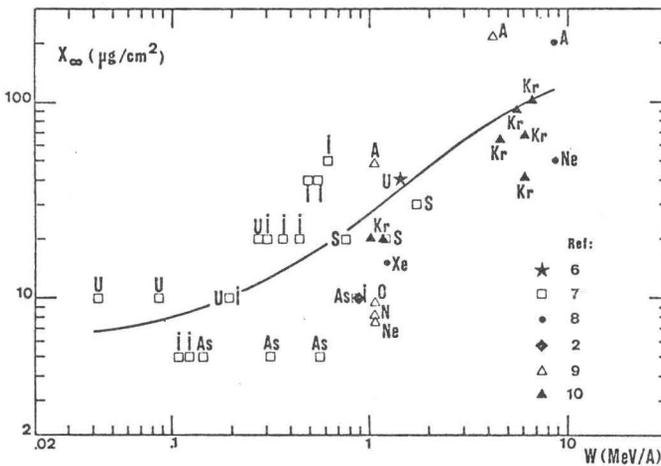
Figure 1 Stripper equilibrium thickness versus beam energy. The projectiles are indicated.
