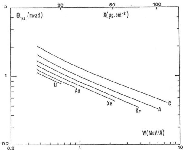
Figure 3 Calculated width (HWHM) of the angular distribution of various ion beams traversing a carbon foil with equilibrium thickness versus energy.
