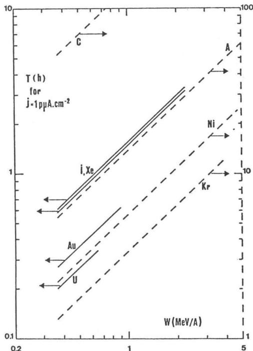
Figure 6 Estimated carbon foil average lifetime under bombardment by various  $1 \mu\text{A} \cdot \text{cm}^{-2}$  ion beams.
