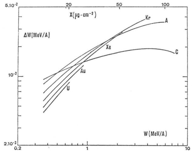
Figure 2 Energy loss of various ions in a carbon foil with equilibrium thickness versus energy.
