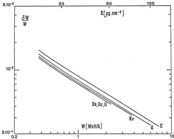
Figure 5 Estimated relative energy spread (HWHM) of various ion beams passing through an equilibrium thickness of carbon.
