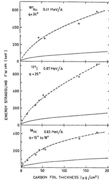
Figure 4 Experimental width (FWHM) of the energy distribution of Au, I, and Ni ions after traversing a carbon foil. From reference (4).
