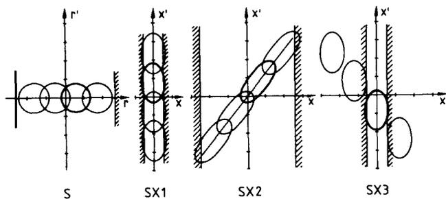
Fig. 2. Schematic diagram of the horizontal (=radial) phase space distribution at the septum S, monochromator entrance slit SX1, divergence limiting slit SX2, and energy analysing slit SX3. The dispersion is indicated by 4 incoherent phase ellipses at slightly different energies. The "hot spot" is marked by a heavy line. Scale divisions are in 1 mm and 1 mrad respectively.
