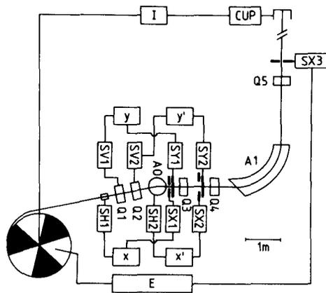
Fig. 1. The closed-loop control systems for the stabilization of the external cyclotron beam.  $x$ -horizontal position,  $x'$ -horizontal direction,  $E$ -energy,  $y$ -vertical position,  $y'$ -vertical direction,  $I$ -intensity
