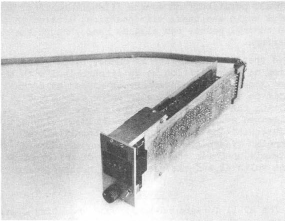
Fig. 2. One of the modular control heads with digital readout, thumbwheel switch and optical rotary encoder.
