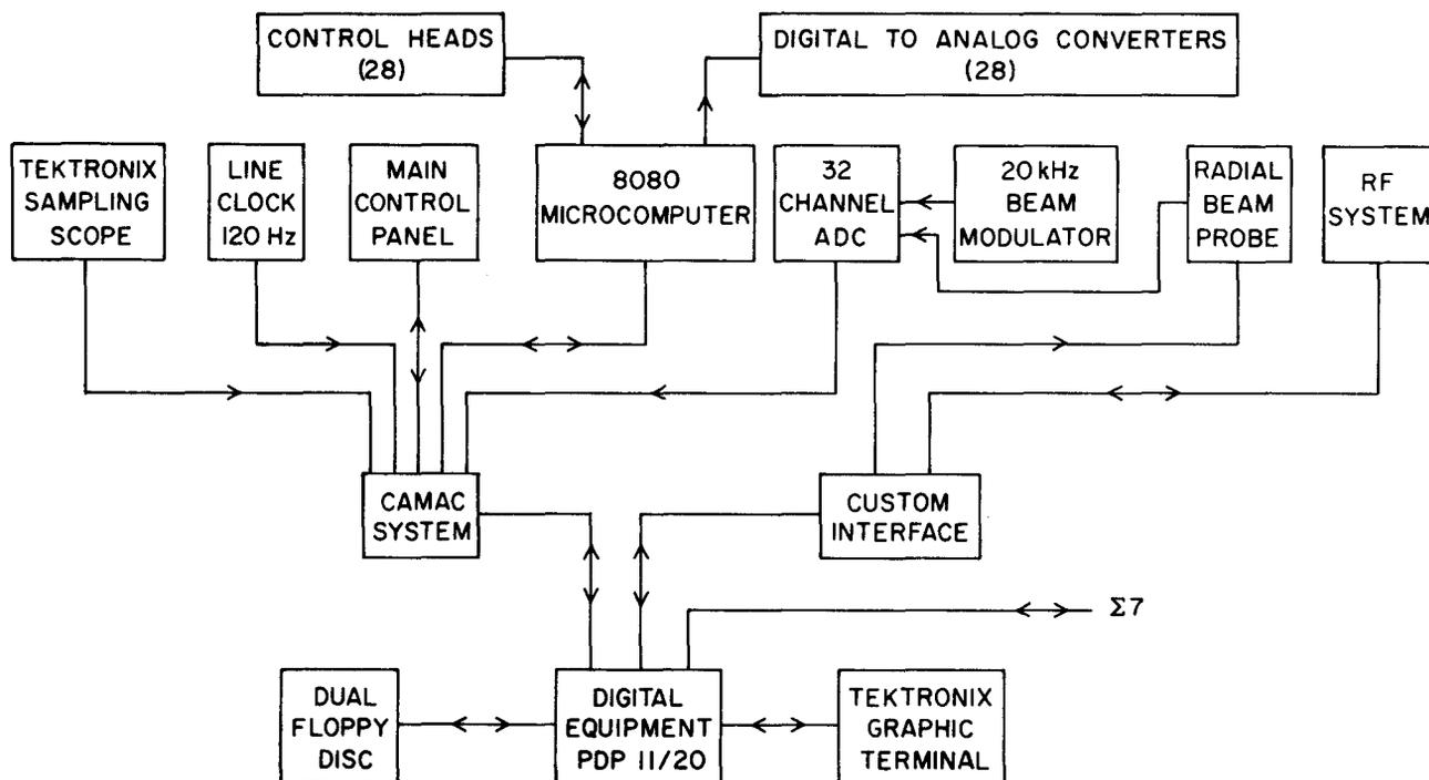
Fig. 1. Block diagram of the cyclotron control system.
