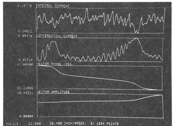
Fig. 5. Same as Fig. 4, but with maladjusted centering controls. Note the effect of radial beam oscillations in the vector phase plot.
