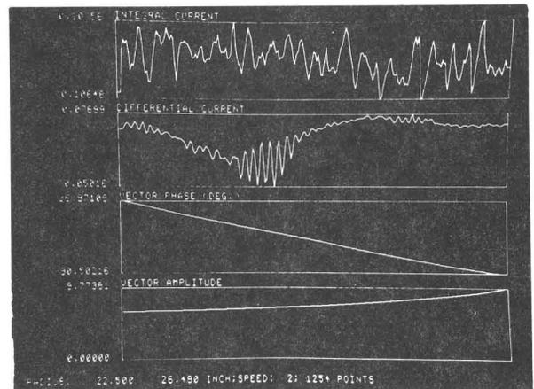
Fig. 4. Radial probe trace shows the integral beam current, the differential beam current and the phase and amplitude of the 20 kHz beam modulation (42 MeV α-particle, 11 μA beam intensity).
