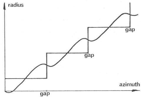
Figure 2 : Accelerated orbit with minimum oscillation in a two gap or two dee geometry.
