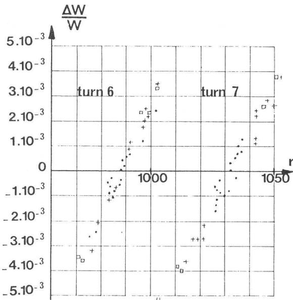
Figure 1 : Simulated  $r-\Delta W$  distribution of the particles after 6 and 7 turns. At such a place, it is possible to cut down the bunch length from  $\pm 7.5^\circ$  to  $\pm 3^\circ$  with a slit or a target between two turns
