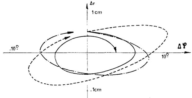
Figure 5 : Motion of a particle in a  $\Delta \varphi - \Delta r$  plane obtained from a stroboscopic view at periodic points showing the effect of the parameter  $A$ . Here the initial values of  $A$  are :
