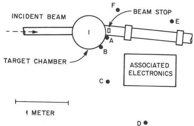
Figure 1. Experimental layout of heavy ion time-of-flight target station at ORIC. The approximate locations are indicated for the fast neutron dose rate readings listed in Table I.
