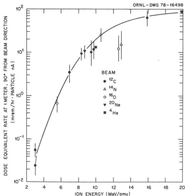
Figure 2. Fast neutron equivalent dose rates one meter from thick targets and 90 degrees from the incident heavy ion beam direction. The targets are iron, nickel, or copper. The curve is drawn to guide the eye. One particle nanoampere is  $6.25 \times 10^9$  particles/second.
