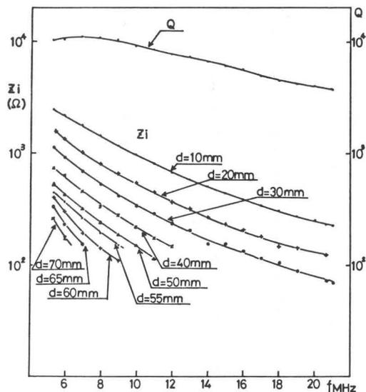
Fig.2 Measured Q values and load impedances versus resonance frequencies for several coupling conditions. "d" is the space between the coupling electrode and the dee electrode.
