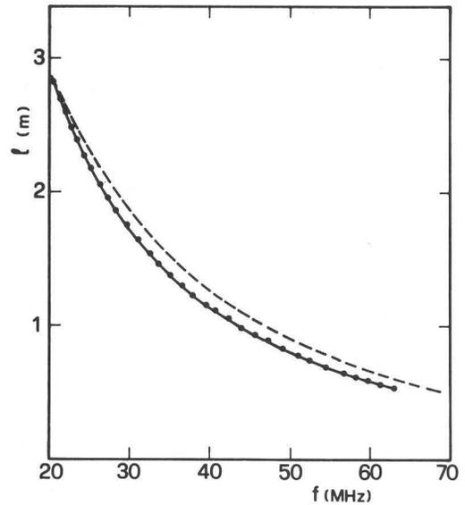
Fig. 5 - Short circuit position as a function of the resonating frequency for the 1:1 model. Dashed line refers to calculated values, points to experimental ones.
