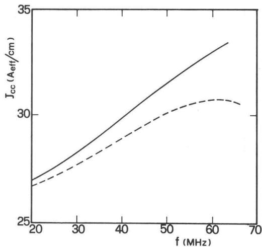
Fig. 7 - Current density at the short circuit, as a function of frequency. Solid line: derived from model measurements. Dashed line: theoretical prediction.
