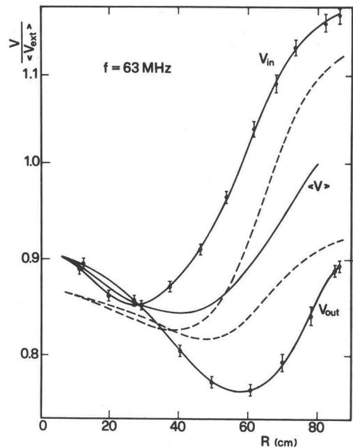
Fig. 9 - Voltage distribution along the dee radius, at 63 MHz. Experimental values (solid lines) and predicted ones (dashed lines) are shown.
