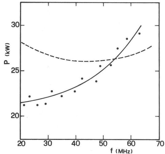
Fig. 6 - Power needed in the cavity, as a function of frequency. Solid line: derived from model measurements. Dashed line: theoretical prediction.
