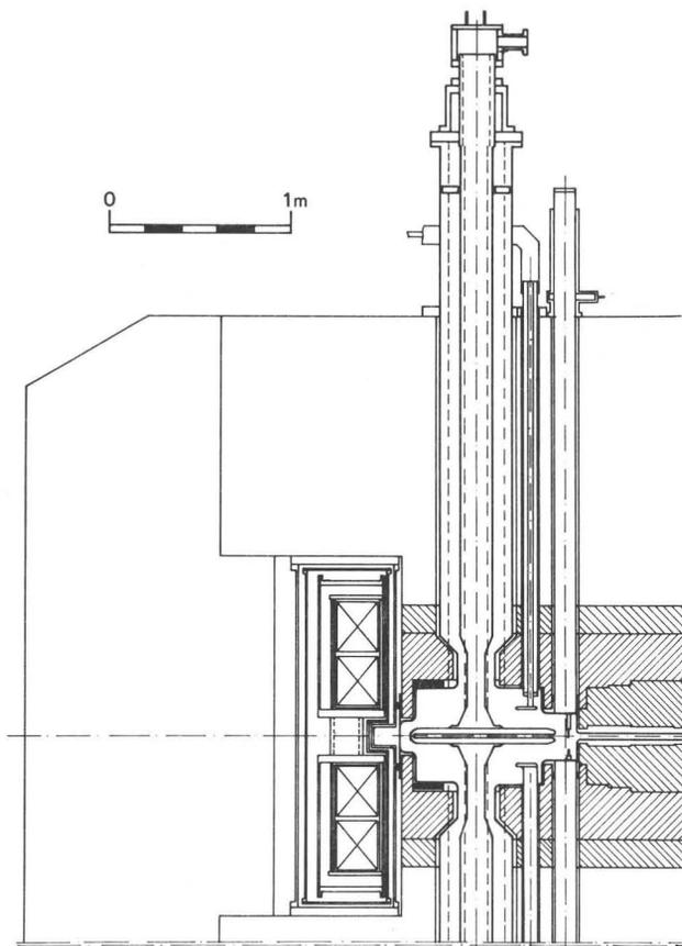
Fig. 11 - Possible improved design of the RF cavity. (see text for details)
