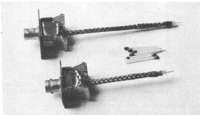
Fig. 8 - Picture of two probes used for voltage distribution measurements along the dee gaps.
