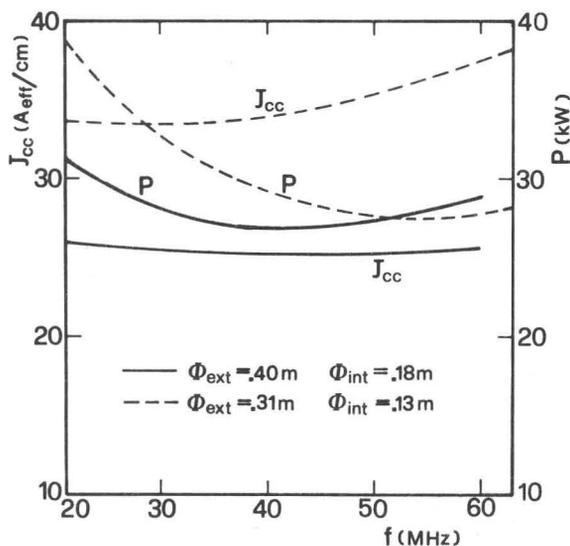
Fig. 12 - Solid lines: short circuit current density and total power in the cavity for the design of fig. 11, with tapering of the coaxial line. Dashed lines: short circuit current density and total power in the cavity for the design of fig. 11, with uniform diameter of the coaxial line (dashed lines in fig. 11).
