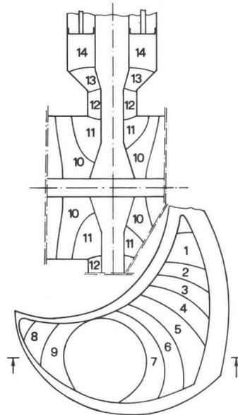
Fig. 1 - Schematic subdivision of the cavity in constant impedance line segments.
