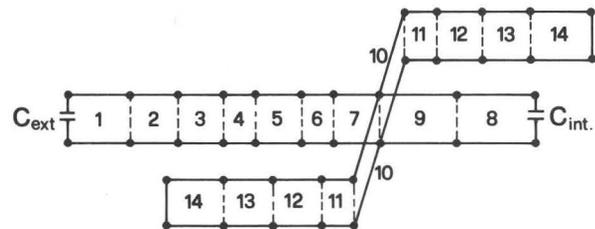
Fig. 2 - Electrical equivalent scheme of the cavity according to the subdivision of fig. 1.
