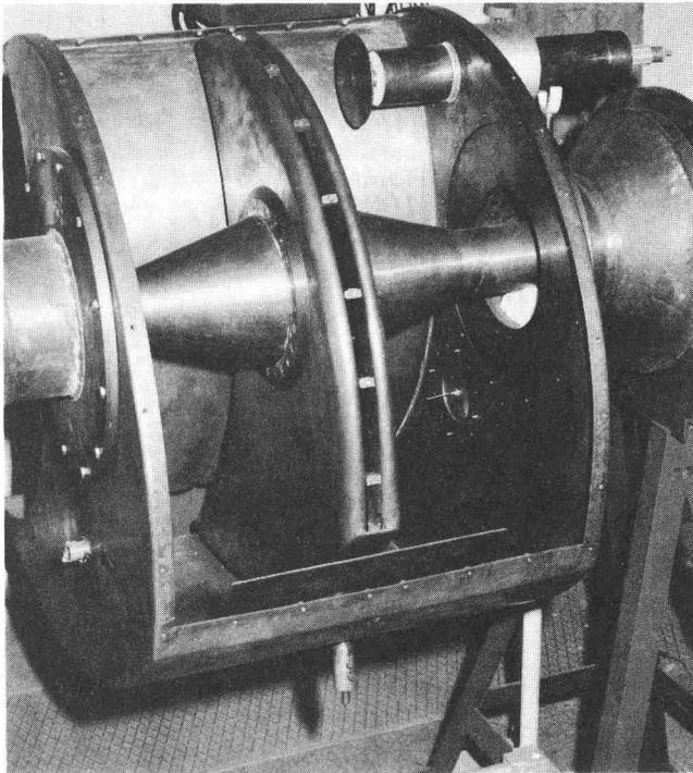
Fig. 4 - Close-up view of the dee and cavity in the model.
