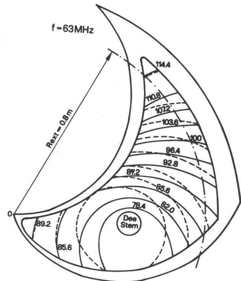
Fig. 10 - Propagation surfaces on the dee, at 63 MHz. Solid lines represent contours derived from model measurements, dashed lines predicted contours.
