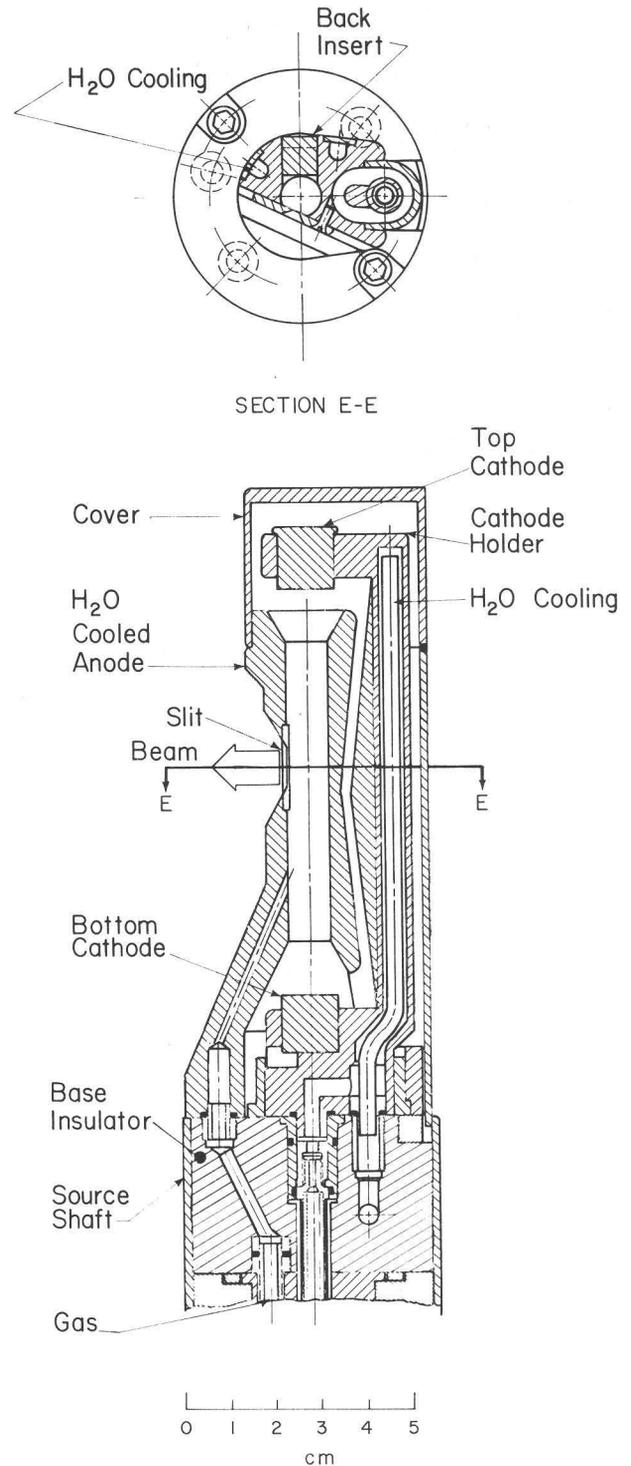
Fig. 1. Schematic cross section of the internal PIG source of the 88-Inch Cyclotron. The anode shown has a 9.4 mm diameter bore and was used for the Li and Be beams reported in this paper.
