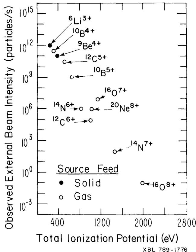
Fig. 3. Observed external beam intensities for 20-32 MeV/nucleon heavy ion beams are plotted as a function of total ionization potential.
