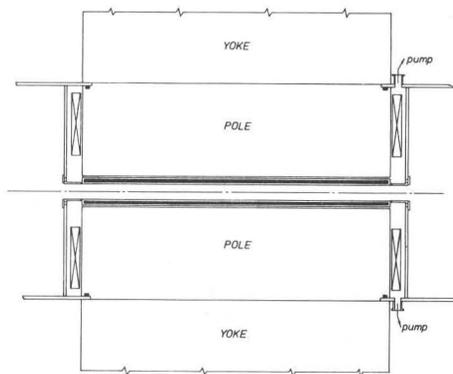
Fig. 4: Chamber design with poles in rough vacuum
