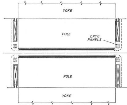
Fig. 2: Chamber design with poles completely in high vacuum.
