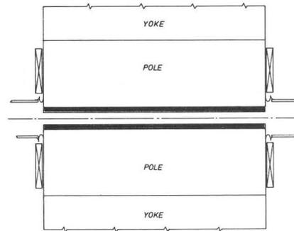
Fig. 3: Chamber design with poles partly in high vacuum.
