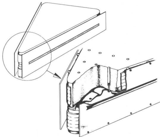
Fig. 6: Assembly of the chamber with the pole pieces
