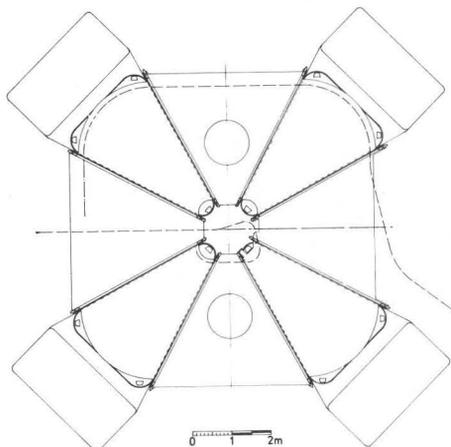
Fig. 1: Octagonal structure of the vacuum vessel for the SSC
