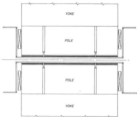
Fig. 5: Chamber design with poles in air and using short bolts for support
