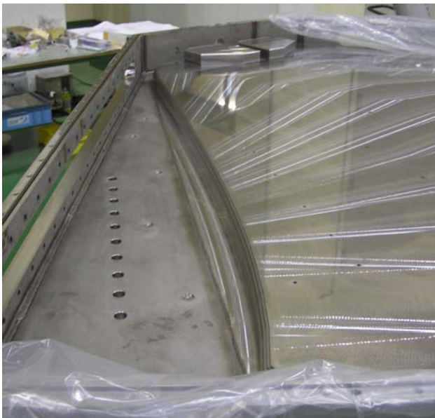
Figure 2: Pole surface of the sector magnet.
