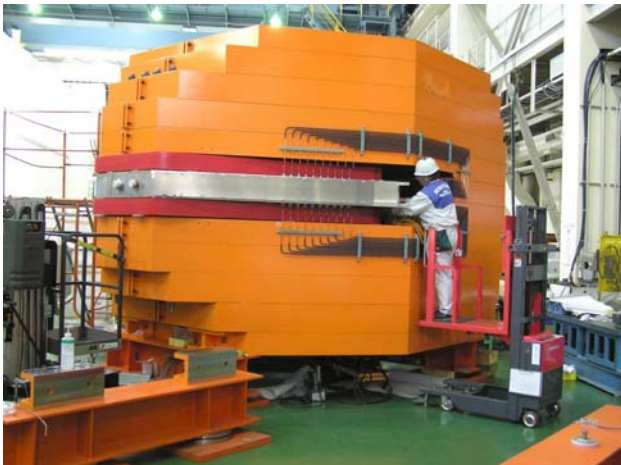
Figure 3: Sector magnet of the fRC under construction.
