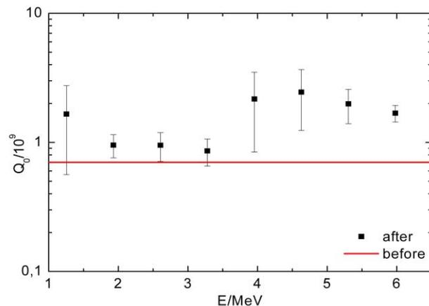
Figure 4: Measured quality factor before and after the heat treatment.
