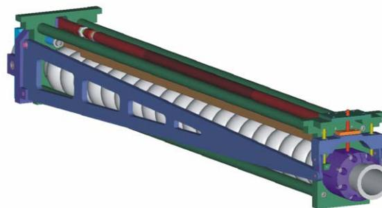
Figure 6: Isometric view of the cavity tuner. The frequency change is provoked by pushing or pulling on the cavity cut-off tubes. The cavity in between is not supported nor hindered in its movement.
