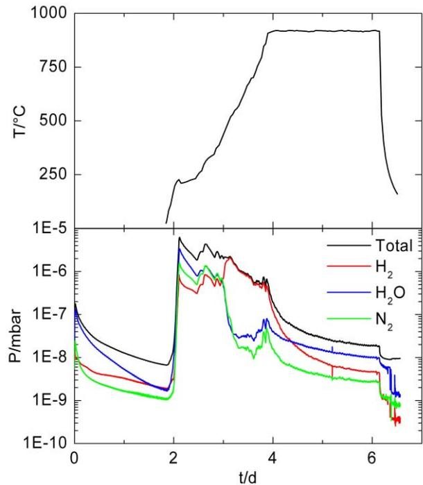
Figure 3: Temperature and partial pressure of the residual gas inside the furnace during the firing procedure. At 300 C hydrogen becomes dominant indicating a huge reservoir.
