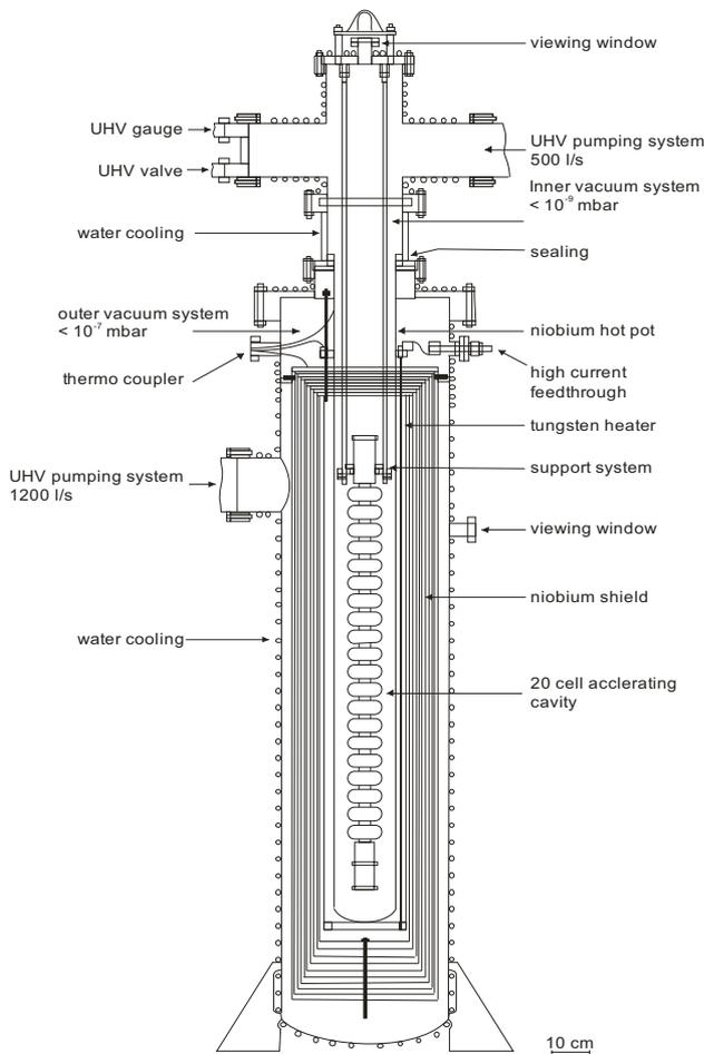
Figure 2: Side view of the UHV furnace originally built and operated in Wuppertal[5], now relocated to Darmstadt.
