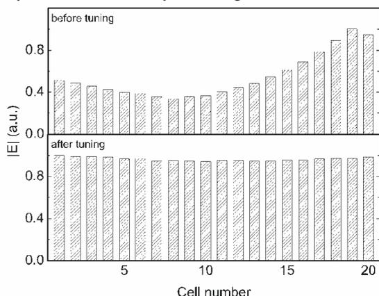
Figure 5: Measured field flatness of one cavity being in operation for more than 10 years. The heavily distorted field profile could be restored during the tuning procedure.
