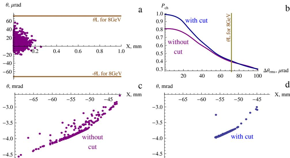
Figure 3: Beam extraction from the Recycler Ring: phase space at the 1<sup>st</sup> crystal entrance (a), the channeling efficiency vs R.M.S. incident angle (b), phase spaces of the extracted beam without cut (c) and with cut (d). Crystal parameters: (110) silicon crystal of 1mm length and thickness, deflection angle 0,5mrad.
