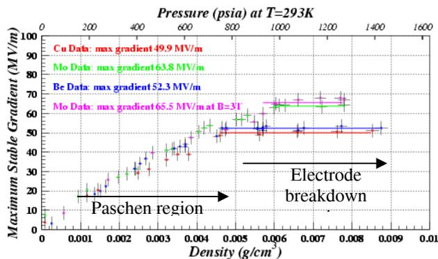
Figure 5: Measurements of the maximum stable RF gradient as a function of hydrogen gas pressure at 805 MHz with no magnetic field for three different electrode materials: Cu (red), Mo (green), and Be (blue). The cavity was also operated at the same gradients in a 3T field with Mo electrodes (magenta).
