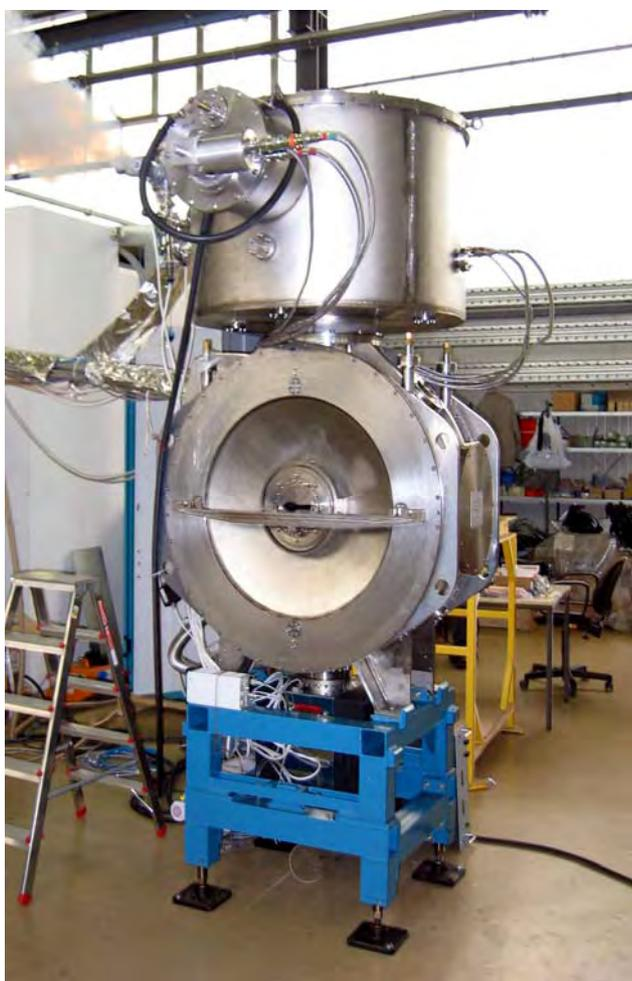
Figure 4: Photo of assembled Superbend cryostat.
