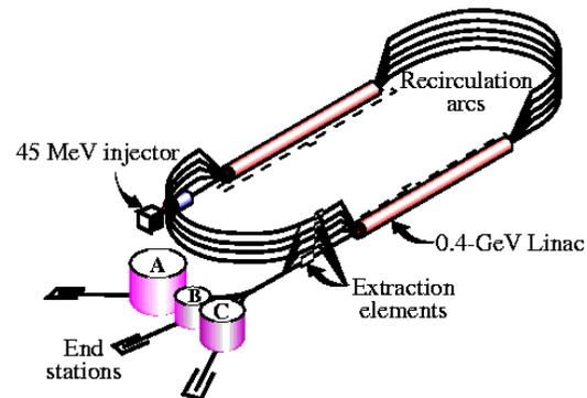
Figure 1: The accelerator is naturally divided into the segments between branch points occupied by the beam on its path to the experimental halls.
