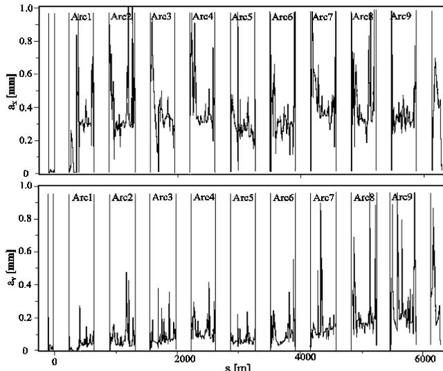
Figure 1. Normalized betatron amplitude for horizontal and vertical beam motion throughout the accelerator in the case of horizontal kick at the beginning of ARC1.
