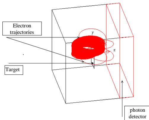
Fig 3. Trajectories of electrons in axial-symmetric magnet field, setup box is  $100 \times 100 \times 100 \text{ cm}^3$  (big gap)
