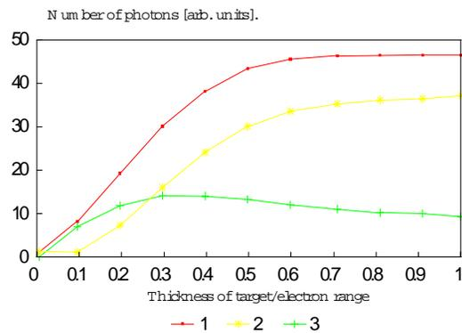
Fig. 1 1- the total number of X-ray photons produced in W-target with depth, 2- the number of X-ray photons absorbed with depth, 3 - the number of surviving X-ray photons.
