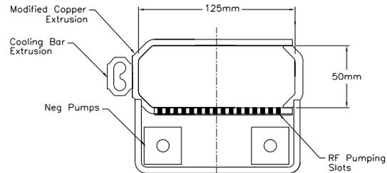
Figure 1. Cross-section of the HEB IR Chamber
