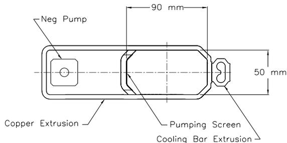
Figure 3. Cross-section of the LEB IR Chamber
