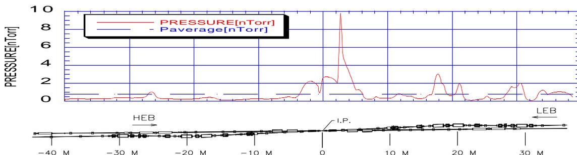
Figure 5. Interaction Region Plan and Pressure Profile
