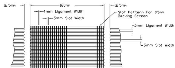
Figure 2. HEB IR pumping slots
