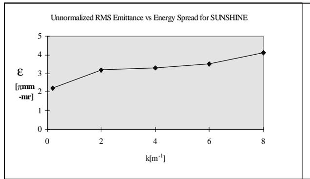
Figure 4: Plot of unnormalized RMS emittance vs. energy spread for SUNSHINE. The energy of the beam was 3.1[MeV] for all measurements.
