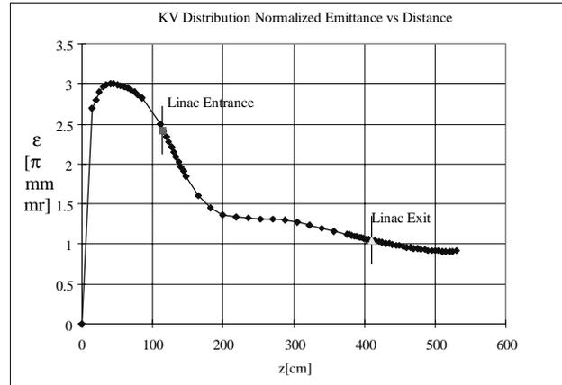
Figure 2: Plot of normalized emittance vs. distance along the GTF for the KV distribution from PARMELA.
