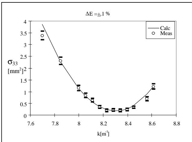
Figure 3: Plot of measured and calculated  $\sigma_{33}$  versus quadrupole strength for the SUNSHINE facility. Where  $\sigma_{33}$  is the square of the vertical beam size.
