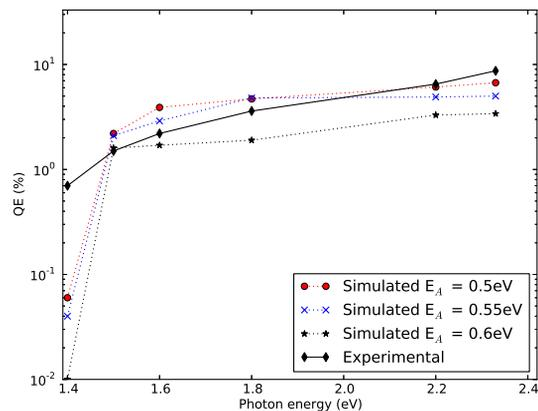
Figure 2: Comparison of measured and simulated spectral response. The electron affinity is an input parameter in the simulations. Results close to the experimental data are obtained for  $\chi = 0.55$  eV.
