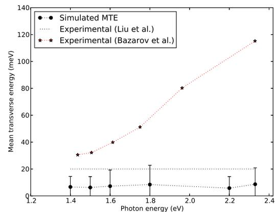
Figure 3: Comparison of measured (Liu *et al.* [10] and Bazarov *et al.* [11]) and simulated MTE using  $\chi = 0.55$  eV in our simulations.
