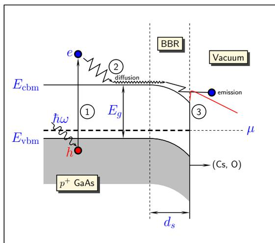
Figure 1: Schematic representation of the three-step model. First, a photon is absorbed causing the generation of an electron-hole pair. Next, the free electron undergoes phonon scattering and diffuses towards the GaAs cesiated electron affinity surface. In the final, third step, a conduction band electron undergoes emission (over barrier or tunneling) or reflection when impinging on the GaAs-vacuum interface.
