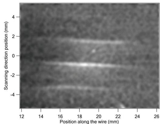
Figure 3: Three images of a wire captured on a single camera frame during a scan. The wire is moving at 20 m/s in the upward direction.
