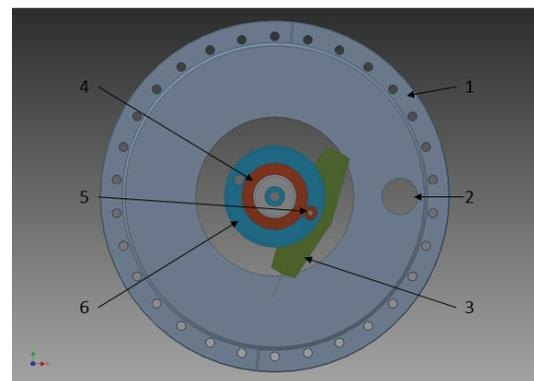
Figure 1: A 3D rendering of the gears setup. (1) - vacuum flange; (2) - beam pipe; (3) - blade with attached carbon wire; (4) - stationary gear  $G_1$ ; (5) - rotating gear  $G_2$ ; (6) - rotating gear box.
