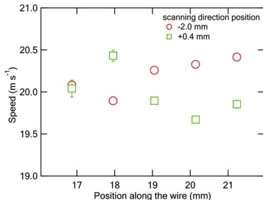
Figure 4: Wire speeds calculated at different locations along the adjacent wires shown in Fig. 3. The circles represent values calculated using the top and middle wires, while the squares use the middle and bottom wires. The error bars are smaller than the symbol size for some points.
