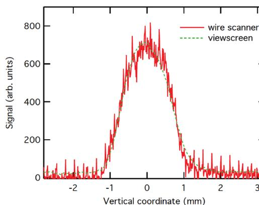
Figure 6: Comparison of the beam profile obtained with the wire scanner (solid line) and the luminescent viewscreen (broken line) for  $20\mu\text{A}$  average beam current (0.015 pC bunch charge).
