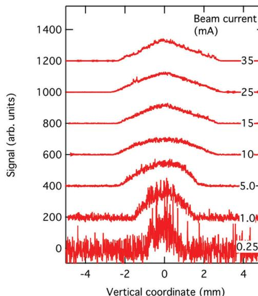
Figure 5: Wire scans at different beam currents, where the data is normalized to 1 mA current.
