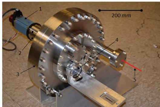
Figure 2: A photograph of the wire scanner. (1) - stepper motor; (2) - ferrofluidic rotary feedthrough; (3) - vacuum flanges; (4) - vacuum flange with viewports; (5) - beam direction.
