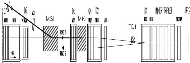
Figure 1: Schematic plan view of IP2 injection
