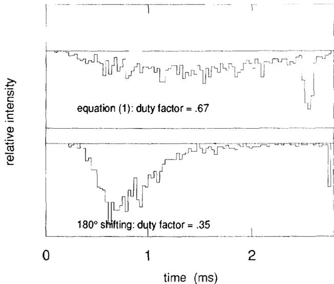
Figure 4. Simulated RF extraction using phase shifting as given by equation (1) and using 180 degree/continuous shifting.
