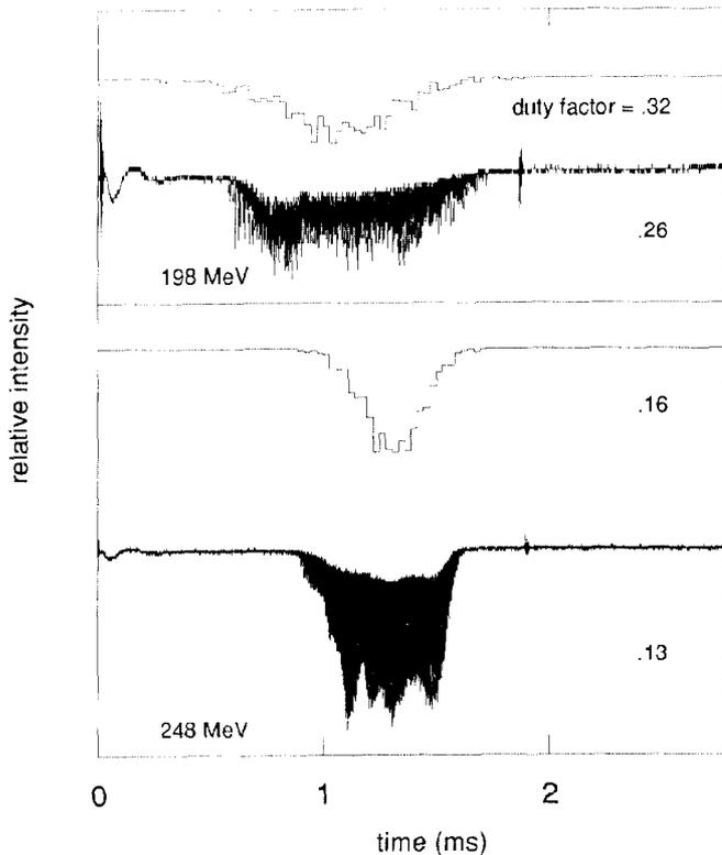
Figure 3. Theoretical and observed extraction at 200 and 250 MeV.
