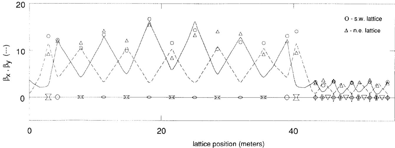
Figure 1. Theoretical betatron functions and measured maxima.
