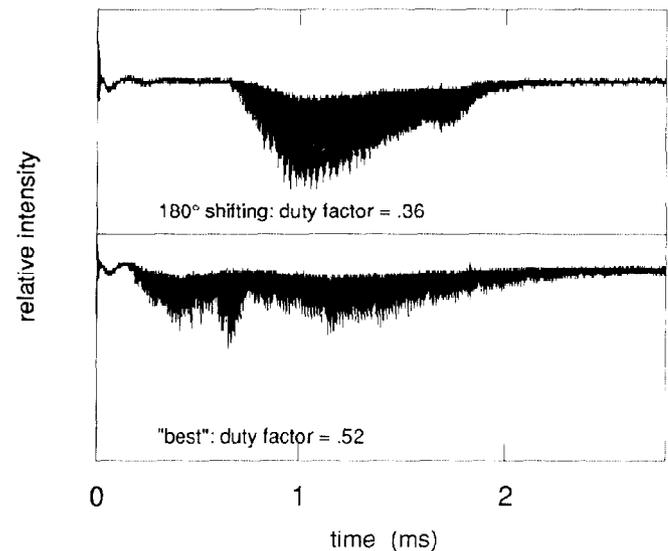
Figure 5. Observed RF extraction at 250 MeV.
