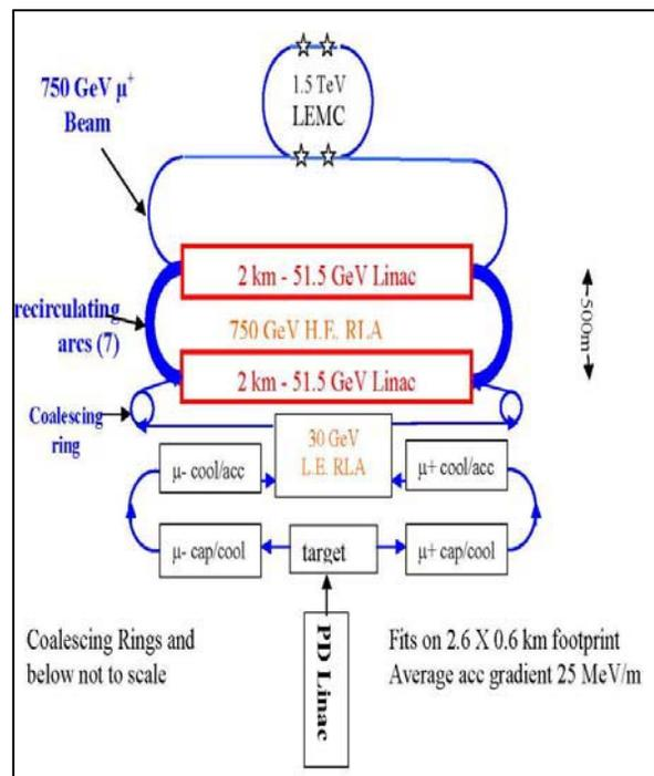
Fig. 1: Schematic layout of a low-emittance muon collider based on a low energy and a high energy recirculating linear accelerator (RLA), showing coalescing rings.
