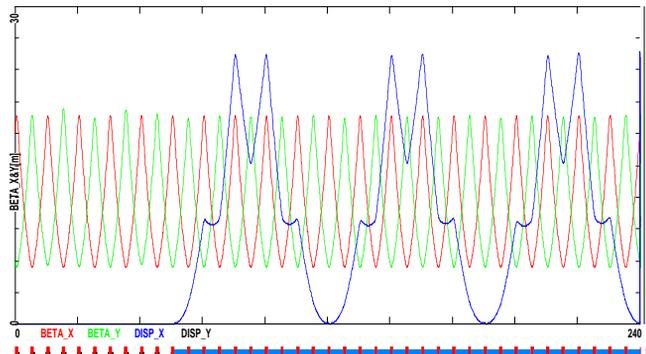
Figure 4: Half of the Racetrack lattice – 5 dispersion free empty cells and 3 Super-periods.
