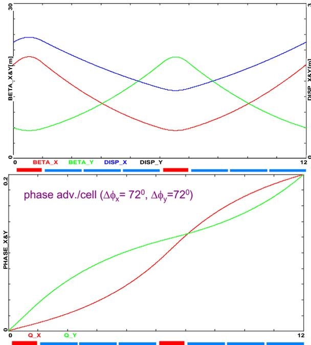
Figure 2: Periodic FODO cells with 72 deg. betatron phase advance in both planes (1.5 meter, 1.6 Tesla dipoles – blue: 1 meter, 14 Tesla/m quadrupoles – red)
