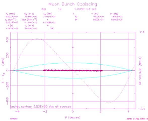
Figure 1a: the distribution of bunches after injection into the coalescing ring
