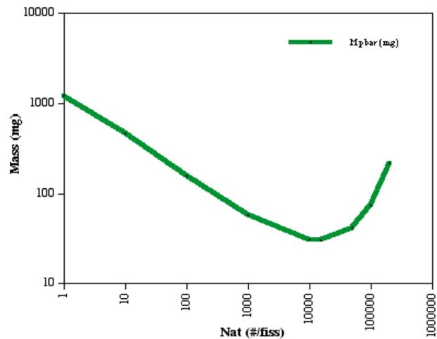
Figure 4: Calculation of the effect of the stored antimatter mass required for this mission scenario as a function of the number of uranium atoms ejected per annihilation.
