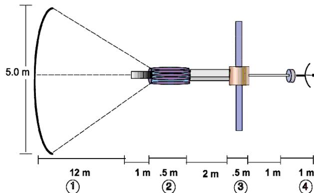
Figure 2: Proposed antimatter driven spacecraft. The primary subsystems are (1) a uranium coated carbon sail, (2) solid H<sub>2</sub>bar crystal storage units, (3) an antiproton driven electrical power supply, and (4) a 10 kg instrument package.
