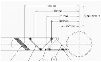
Figure 1: Mechanical schematic of the wire/plate support structure. The thin wire is  $25\mu\text{m}$  in diameter. The thick wire is 1mm in diameter. The plate is 1mm by 10mm. The wire frame is moved into the beam along a  $45^\circ$  axis with respect to the horizontal axis.
