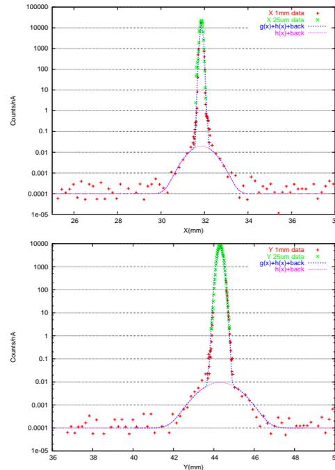
Figure 2: Beam Profile combining the  $25\mu\text{m}$  and 1mm Fe wire data. The top(bottom) plot shows the X(Y) data and results of the fit to the data. The red points represent the 1mm wire data, the green points the  $25\mu\text{m}$  wire data, the blue curve is the overall fit to the data and the red curve is the halo portion of the fit. The ordinate is plotted with a log-scale and the count rate is normalized to the beam current.
