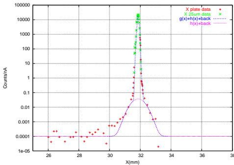
Figure 3: X Beam Profile combining the  $25\mu m$  and  $1 \times 10mm^2$  steel plate data. The red points represent the 1mm wire data, the green points the  $25\mu m$  wire data, the blue curve is the overall fit to the data and the red curve is the halo portion of the fit. The ordinate is plotted with a log-scale and the count rate is normalized to the beam current.
