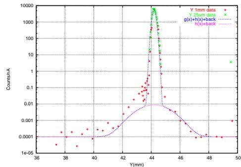
Figure 4: Beam Profile combining the  $25\mu m$  and 1mm Fe wire data. The top(bottom) plot shows the X(Y) data and results of the fit to the data. The red points represent the 1mm wire data, the green points the  $25\mu m$  wire data, the blue curve is the overall fit to the data and the red curve is the halo portion of the fit. The ordinate is plotted on a log-scale and the count rate is normalized to the beam current.
