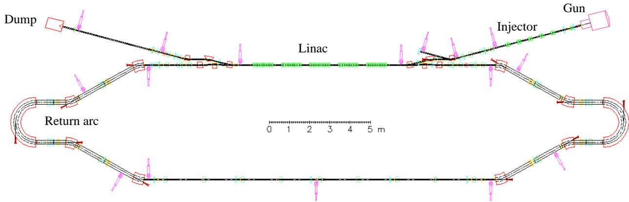
Figure 1: Layout of the Cornell ERL Prototype
