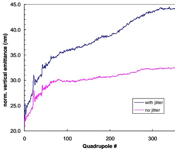
Figure 1: Results of simulating DFS on the TESLA linac (average over 100 seeds). The black line shows results with a stable; the magenta line shows the effects of  $\sim 1\sigma_y$  beam jitter. In both cases BPM noise was included ( $10 \mu\text{m RMS}$ ).
