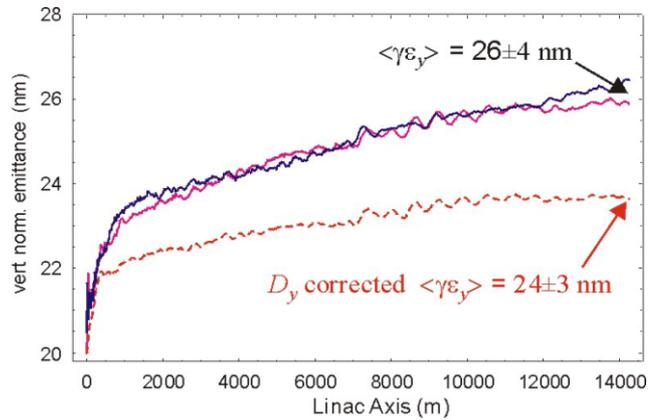
Figure 3: Results of simulations of ballistic alignment for the TESLA linac (averaged over 100 seeds). The two solid lines show independent results from the simulation codes MERLIN [9] (red) and PLACET [7] (blue). The red dotted line shows the emittance after the linear energy correlations are removed.
