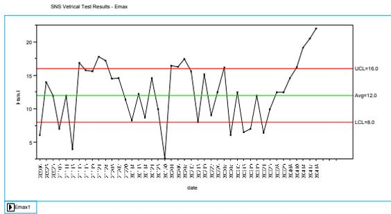
Figure 5. Cavity  $E_{acc}$  Limit Process Chart
