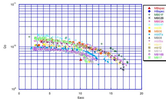
Figure 4. Q<sub>0</sub> vs E<sub>acc</sub> for SNS Medium Beta Cavities
