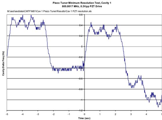
Figure 10. Piezo Tuner Resolution,  $\sim 1$ Hz
