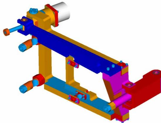
Figure 1. SNS Cavity Tuner Assembly
