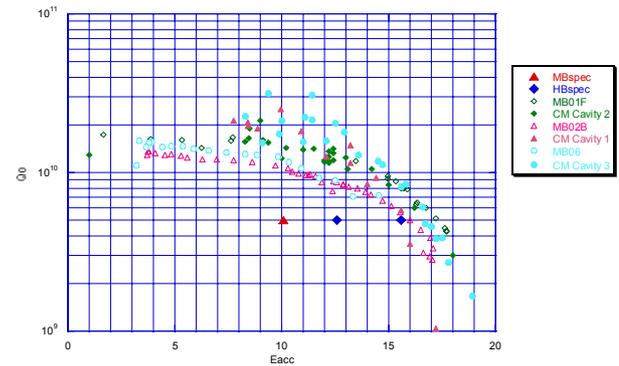
Figure 11. Cavity  $Q_0$  in Final Assembly
