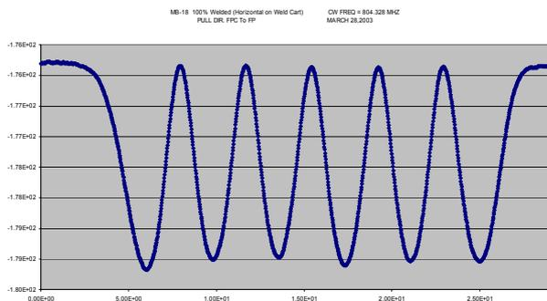
Figure 2. Typical Field Flatness Measurement
