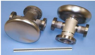
Figure 4: Photograph of 1/2 cell Nb cavity
