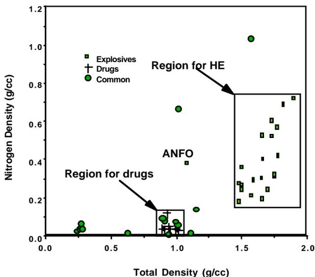
Figure 1: Nitrogen-based High Explosive (HE) identification using the gamma resonance CDS technique [2].
