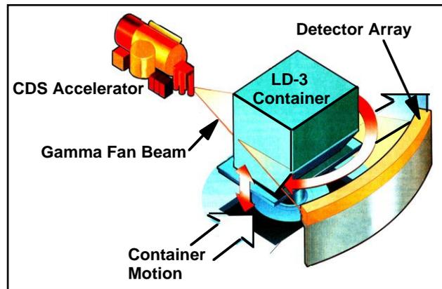
Figure 2: LD-3 airline cargo container CDS interrogation concept [2].
