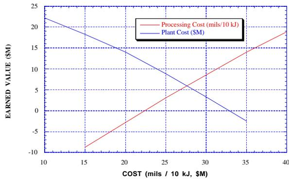
Figure 5: Earned value as a function of plant cost (\$M) and unit processing cost (mils/10 kJ).
