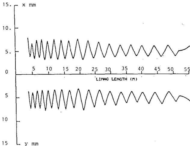
Fig. 5 : Beam envelopes for positrons in Linac W for an emittance of  $4.8 \pi$  mm.mrad. at 600 MeV.
