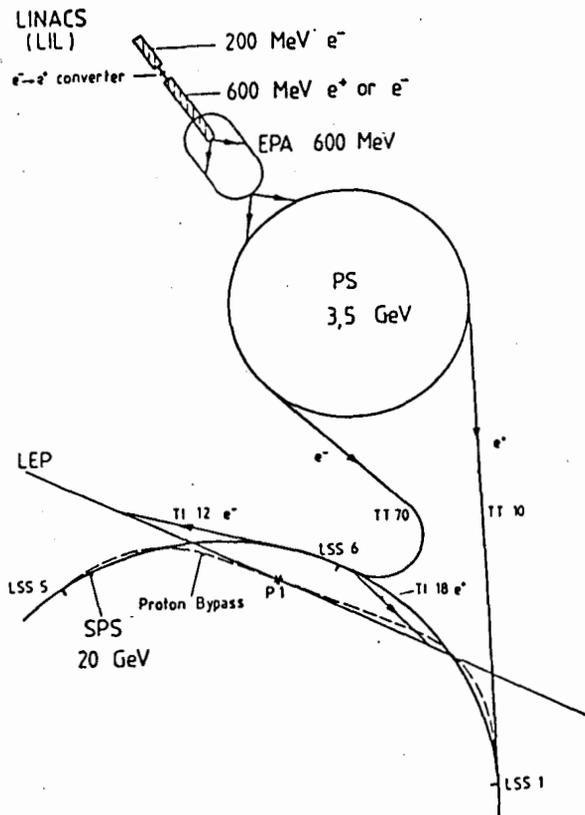
Fig. 1 : Schematic layout of the LEP injector chain. The dashed line indicates the possible future SPS bypass of the ep option. Of LEP, only the part around the crossing point 1 (P1) is shown.
