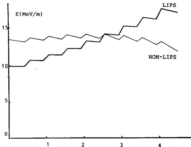
Fig. 3 - Computed acceleration rate versus longitudinal particle position in the LIL TW accelerating section for LIPS and non-LIPS. Main parameters : for non-LIPS as in Table I ; for LIPS Q(spheres) = 150 000,  $\tau_p$  (RF pulse length) = 3,9  $\mu$ s,  $\pi$  phase-switch at  $\tau_p$  minus 1.2  $\mu$ s.
