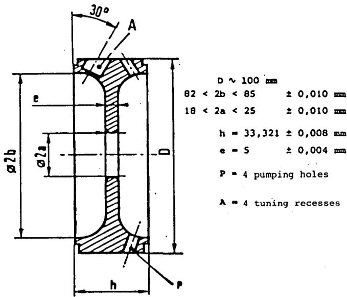
Fig.2: Mechanical features of LIL unit cell.
