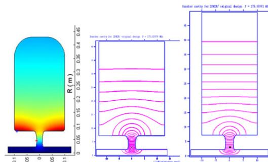
Figure 1: Pillbox re-buncher magnetic (left) [2] and electric (right) field maps.
