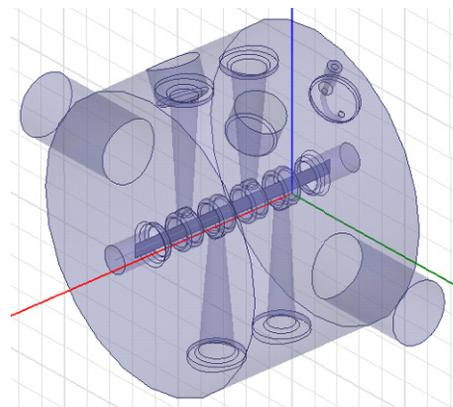
Figure 3: 5-gaps IH cavity.
