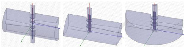
Figure 2: 3 and 4 gap resonators: 3-gap QWR (left), 4-gap QWR (middle), and 4-gap IH (right).
