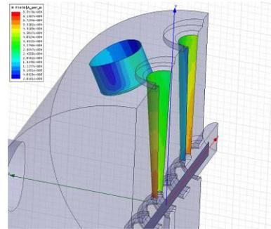
Figure 5: Magnetic field distribution on the tuner.
