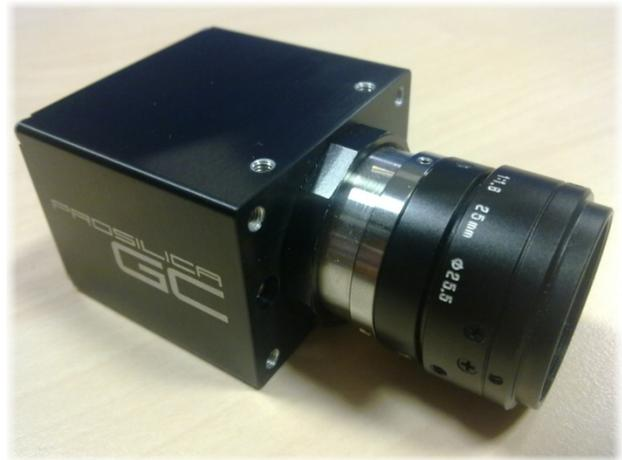
Figure 1: Prosilica GC1020 Camera.
