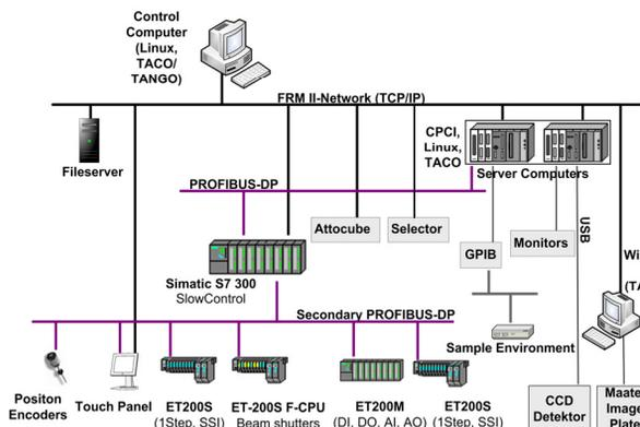
Figure 2: Physical architecture of the BIODIFF control and data acquisition system.
