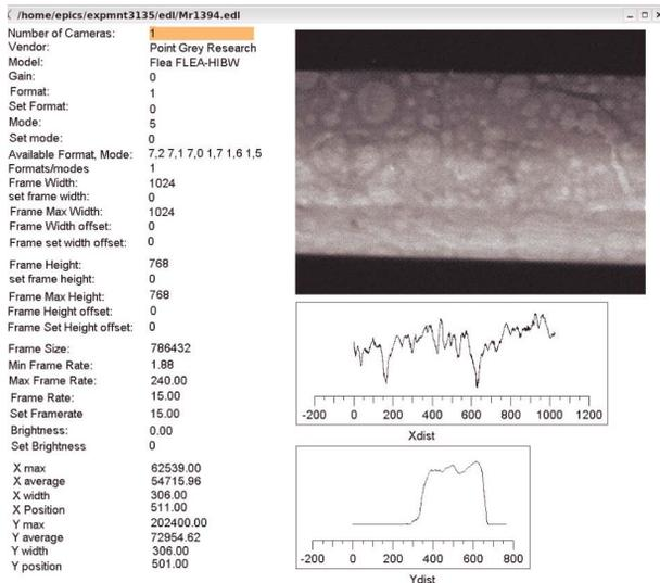
Figure 2: X-ray image of blemishes in the coating of a beryllium window.
