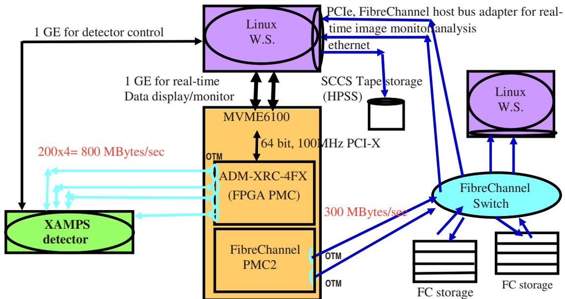
Figure 3: Block diagram of image processing system for testing the XAMPS detector
