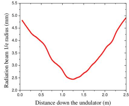
Figure 3: Size of the radiation beam as a function of distance down the undulator.
