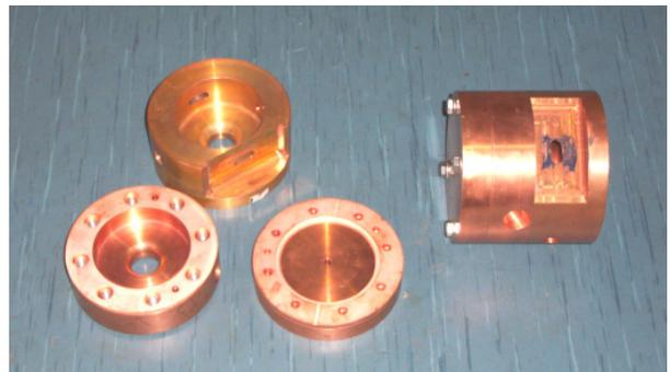
Figure 7: Components of the ETP Cu prototypes of the photocathode RF gun.
