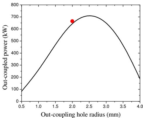
Figure 2: Optimisation curve for the size of the out-coupling hole.
