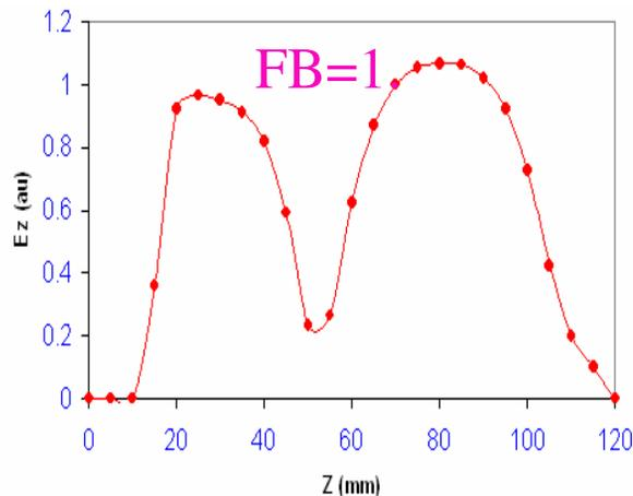
Figure 8: Bead-pull of a tuned Al prototype photocathode gun.
