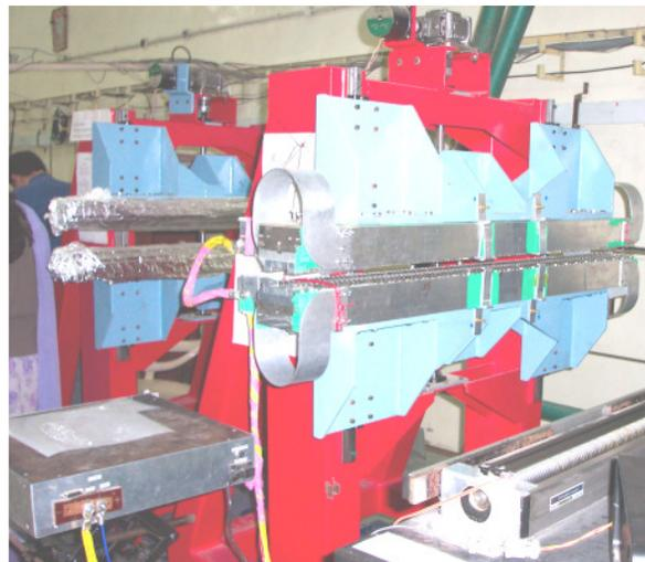
Figure 4: A view of the two undulator segments, each of length 1.25 m.
