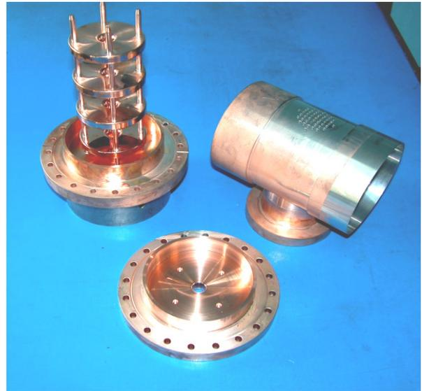
Figure 6: Components of the 4-cell PWT linac structure.
