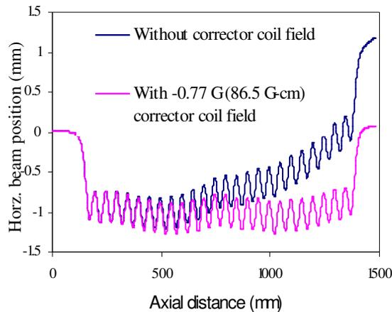
Figure 5: Electron beam trajectory through the undulator, with and without the corrector coil.
