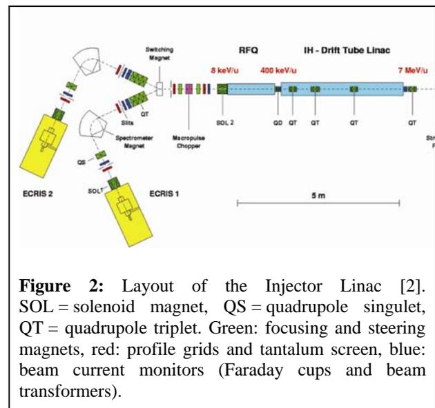
**Figure 2:** Layout of the Injector Linac [2]. SOL = solenoid magnet, QS = quadrupole singlet, QT = quadrupole triplet. Green: focusing and steering magnets, red: profile grids and tantalum screen, blue: beam current monitors (Faraday cups and beam transformers).
