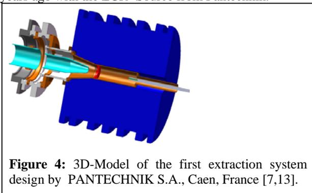
**Figure 4:** 3D-Model of the first extraction system design by PANTECHNIK S.A., Caen, France [7,13].
