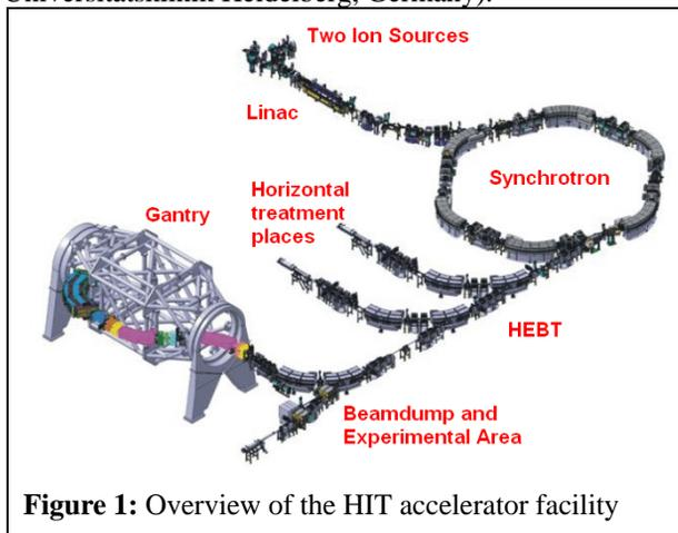
**Figure 1:** Overview of the HIT accelerator facility
