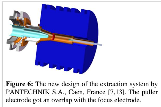
**Figure 6:** The new design of the extraction system by PANTECHNIK S.A., Caen, France [7,13]. The puller electrode got an overlap with the focus electrode.
