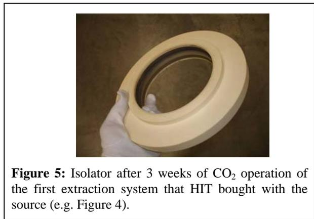
**Figure 5:** Isolator after 3 weeks of CO<sub>2</sub> operation of the first extraction system that HIT bought with the source (e.g. Figure 4).
