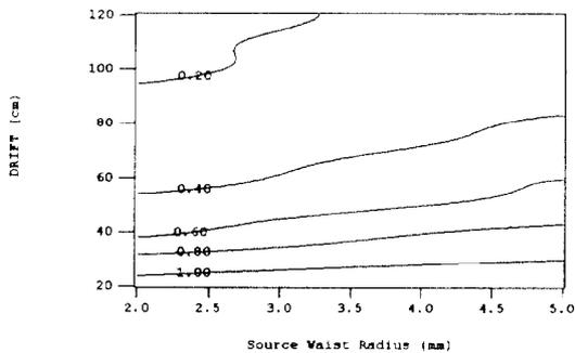
Figure 2. Contours of  $\epsilon_{cnz}/\epsilon_{cnp}$  at each source waist radius and initial drift length for fixed normalized source emittances of  $\epsilon_{snx} = \epsilon_{sny} = 0.365$  mm-mrad for a 3Q injection line.
