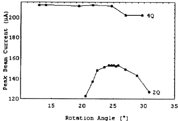
Figure 3. Peaked beam current at the 1 MeV beamstop as a function of 2Q & 4Q axial orientation angle. This experiment was performed on the 1 MeV test cyclotron using a 4.8 ampere source arc current setting.
