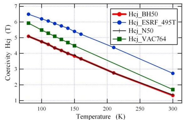
Figure 5: Variation of the coercivity versus the temperature.
