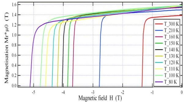
Figure 3: The second quadrant of the hysteresis cycle without the surface effect.
