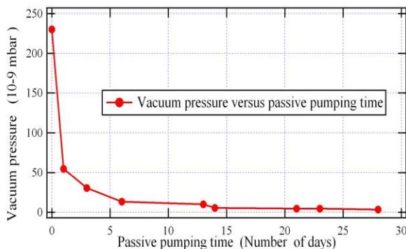
Figure 7: Vacuum pressure versus passive pumping time.
