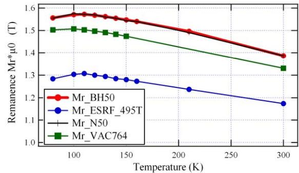
Figure 4: variation of the remanence versus the temperature.
