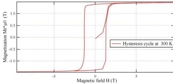
Figure 1: Characterisation of the BH50 at 300 K.
