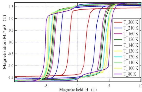
Figure 2: Hysteresis cycle of BH 50 versus temperature.
