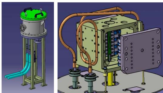
Figure 6: Permanent magnet test bench.
