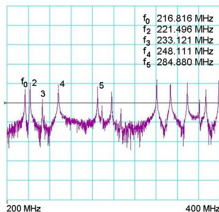
Figure 8: Frequency spectrum of the IH-DTL.
