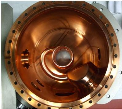
Figure 4: Open debuncher cavity with spiral and drift tube.
