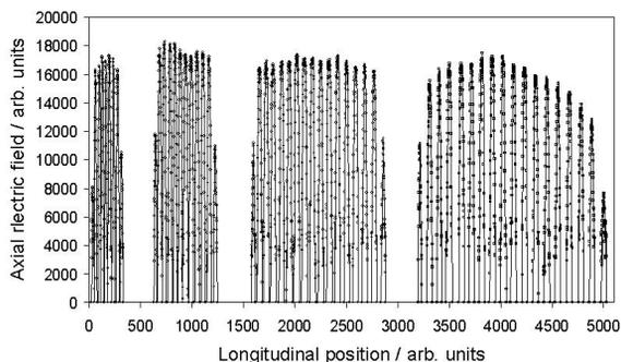
Figure 6: Measured final on-axis electric field distribution. The maximum corresponds to about 18 MV/m.
