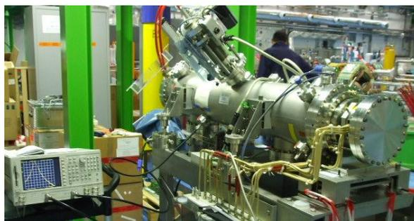
Figure 1: RFQ test bench with CNAO RFQ at GSI.
