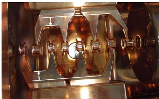
Figure 5: Drift tubes with a higher base (arrows) in section no. 1 (low energy end). To the right, the entrance part of the first internal triplett lens is visible.
