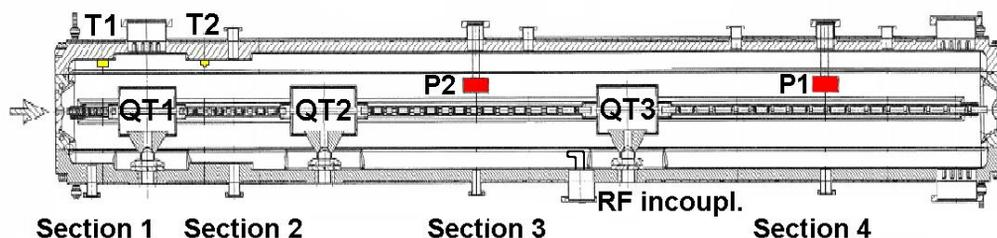
Figure 2: IH-DTL with four KONUS sections, three internal magnetic Quadrupole Triplet lenses (QT1 – QT3), movable RF plungers (red: P1, P2), and inductive tuning plates (yellow: T1, T2). The length of the cavity is about 3.8 m.
