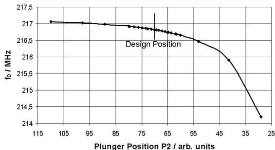
Figure 7: Resonance frequency vs. plunger position.
