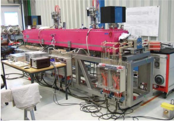
Figure 3: IH-DTL during low level RF tests at GSI.
