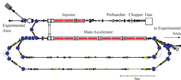
Figure 1: Floor plan of the S-DALINAC.
