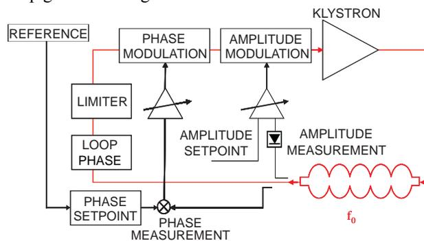
Figure 2: Self Excited Loop diagram.
