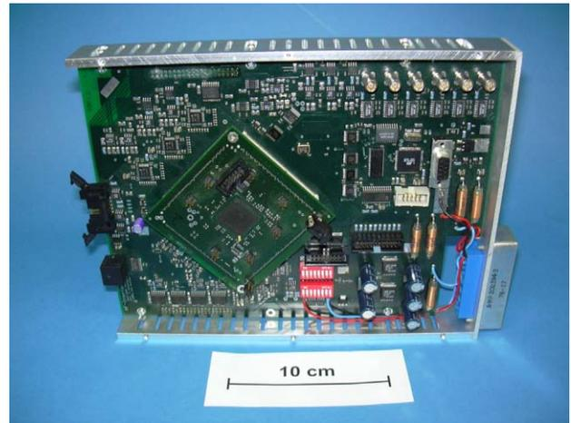
Figure 4: Picture of the FPGA-board's prototype.
