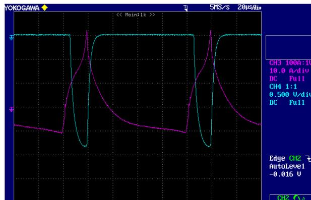
Figure 2: The profile of pulse beam measured at external faraday cup. The blue line is beam profile.
