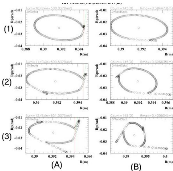
Figure 1: The results of beam tracking. (A) is the beam phase diagram at mass less septum and (B) is at electrostatic septum. (1) is the beam phase diagram at certain turn number near the 500keV beam energy, (2) is at next turn and (3) is at after next turn.
