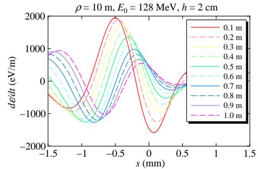
Figure 4: CSR wake with shielding from the end of bending magnet. The shielding chamber height is 2 cm.
