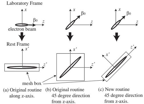
Figure 8: Bounding box sizes in the rest frame for the original GPT space charge mesh routine and the enhanced version.
