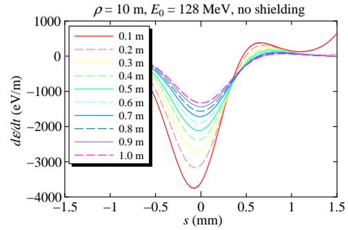
Figure 3: CSR wake without shielding from the end of bending magnet. The bunch length is 0.3 mm.
