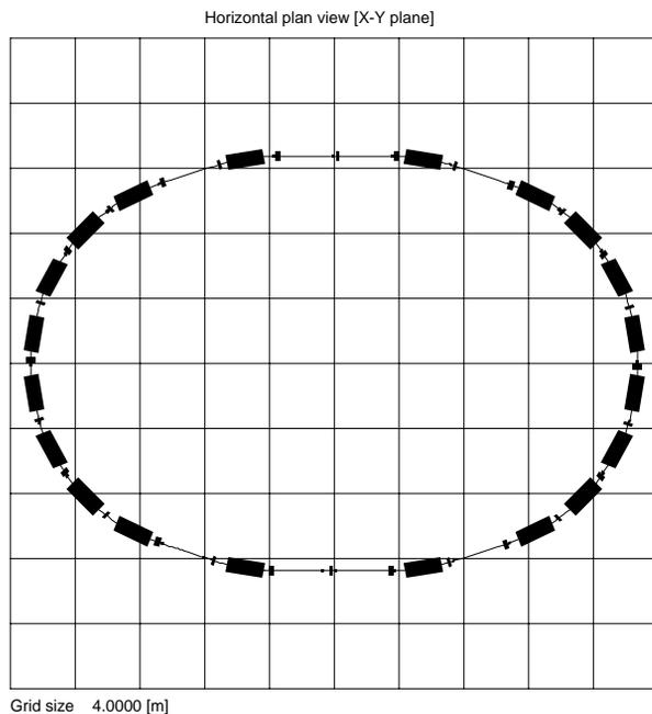
Figure 1. Footprint of the CLS Booster lattice.
