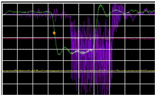
**Figure 4.** Yellow trace: Circulating beam current in the booster synchrotron at 2900 MeV (2 mA/div., 50 ns/div.). Green trace: FCT signal in booster synchrotron (8 mA/div., 50 ns/div.). Purple trace: FCT signal in the BTS transfer line (8 mA/div., 50 ns/div.).
