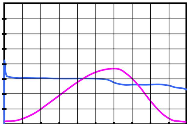
Figure 3. Blue trace: Average circulating beam current in the booster synchrotron throughout the 1 s ramping cycle (4 mA/div., 0.1 s/div.). Red trace: Beam energy.
