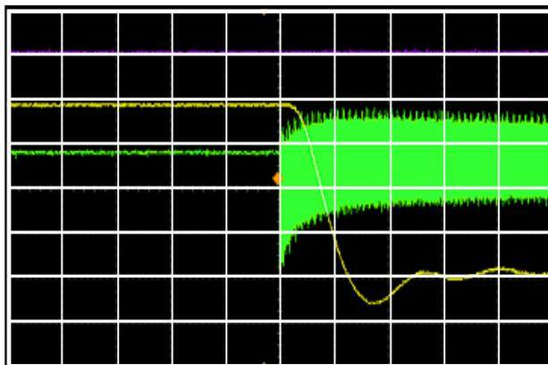
**Figure 6.** Green trace: FCT in booster synchrotron (20 mA/div., 0.1 ms/div.). Yellow trace: DCCT signal in the booster synchrotron with a 1 kHz bandwidth (4 mA/div., 0.1 s/div.).
