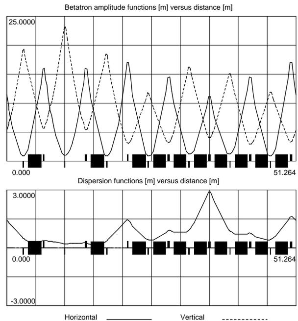
Figure 2. Lattice functions over half the circumference.
