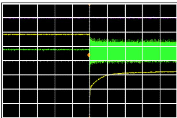
**Figure 7.** Green trace: FCT in booster synchrotron (20 mA/div., 5 ms/div.). Yellow trace: DCCT signal in the booster synchrotron with a 1 kHz band width (4 mA/div., 5 ms/div.).
