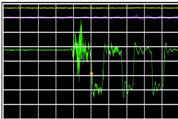
**Figure 5.** Green trace: FCT in booster synchrotron (20 mA/div., 200 ns/div.).
